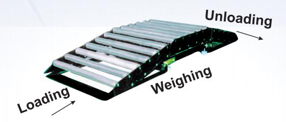
For ease of loading and unloading of carboy and drums filled with chemicals the platform scales are provided with ramps, rollers on the ramps on one side or both the sides and rollers on platform of the scale. Rollers available in M.S. Material with Zinc passivasion or S.S. 202 or S.S. 304 depending on the need.
