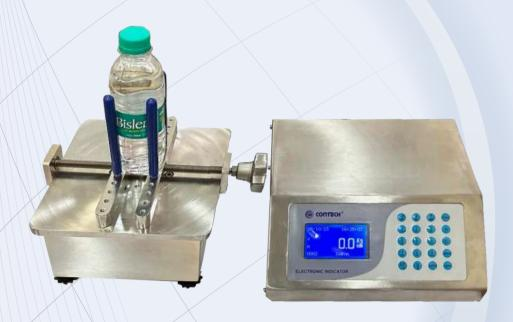
Contech bottle torque tester is used for measuring the torque required to open the cap of bottles.
